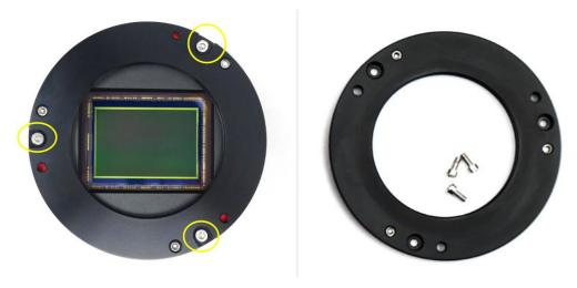
♦ loose the 6 screws which fix the cover, please loose the screws on average
