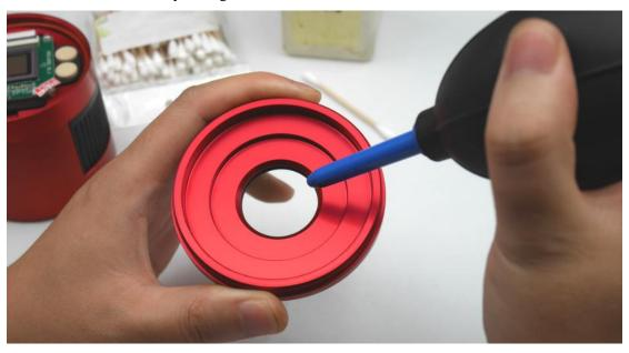
**Step7:** Clean the spots on the inner surface of protective window
